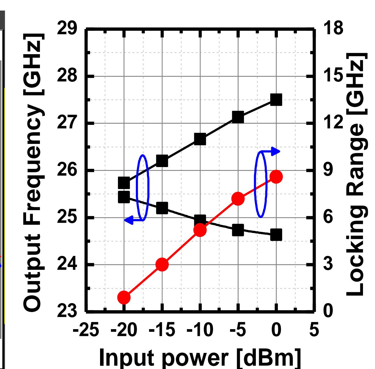
Fig. 10. Measured sensitivity curve and locking range for the proposed ILFD.
