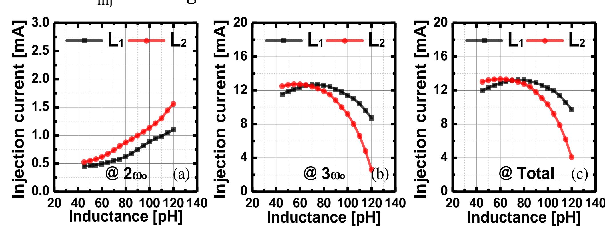
Fig. 4. Injection current at (a)  $2\omega_o$ , (b)  $3\omega_o$ , and (c) total ( $I_{2\omega_o} + I_{3\omega_o}$ ) versus  $L_1$  and  $L_2$ .
