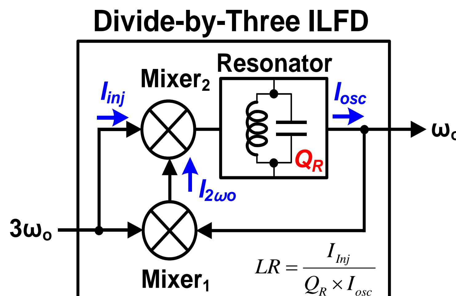
Fig. 1. A block diagram of the function of divide-by-three injection locked frequency divider (ILFD).
