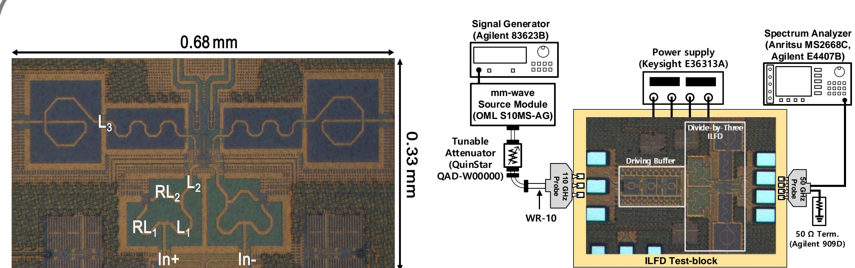
Fig. 7. A microphotograph of the proposed ILFD chip with the inductive feedback (core size: 0.68 x 0.33 mm<sup>2</sup>).
