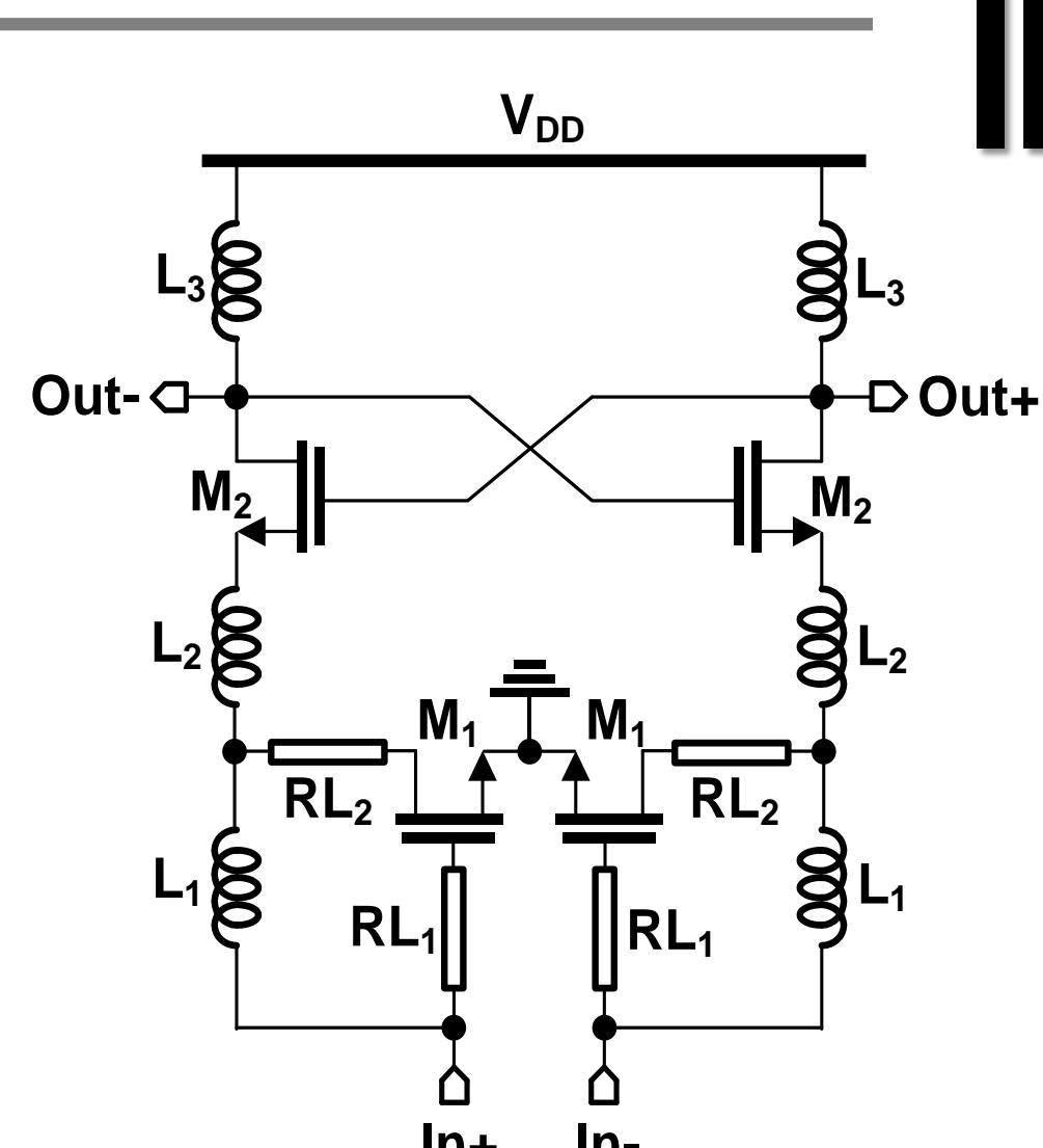
Fig. 2. Schematic of the proposed ILFD with inductive feedback for  $I_{inj}$  boosting.
