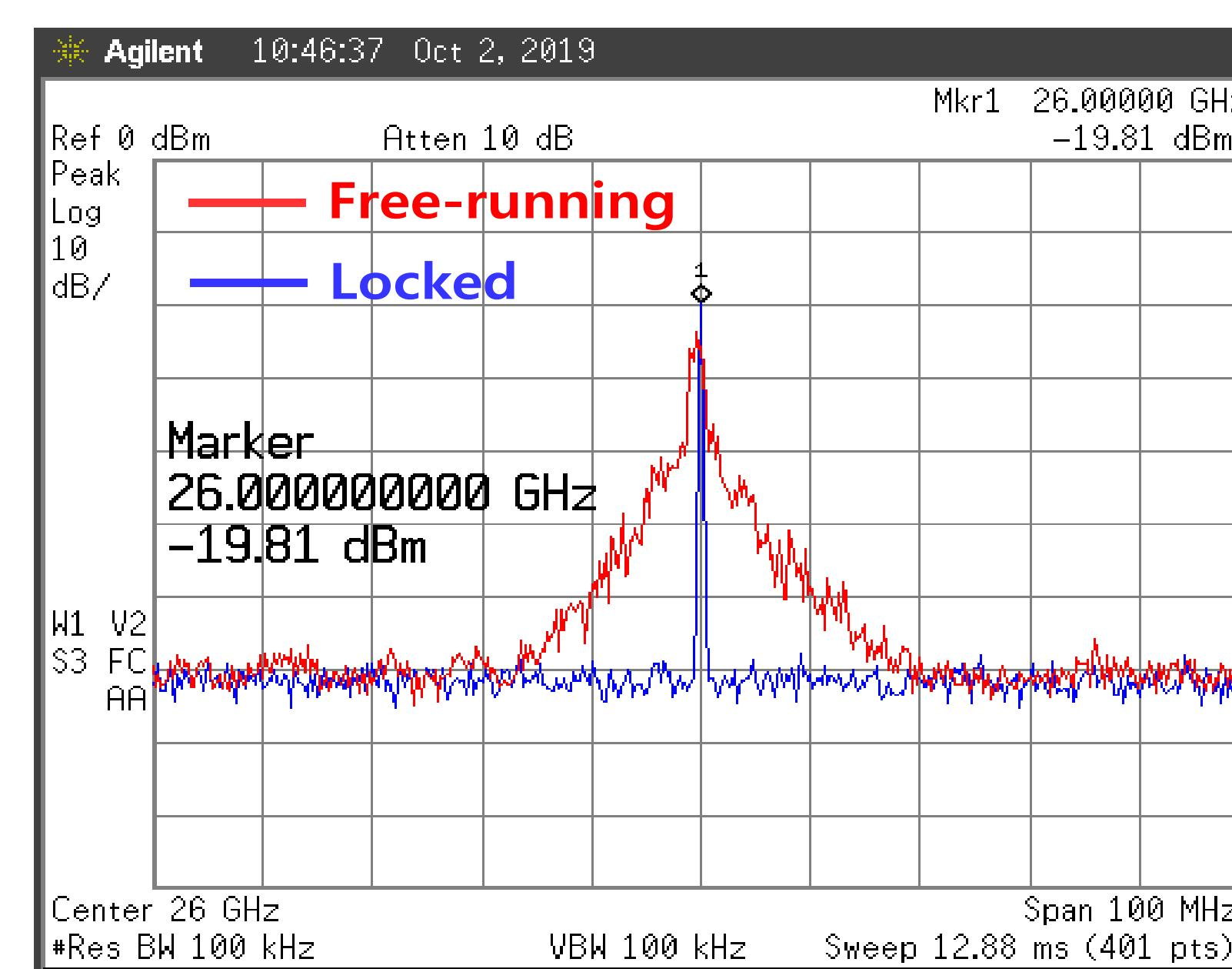
Fig. 9. Measured spectra in free-running and locking state for the proposed ILFD with input frequency of 78GHz.
