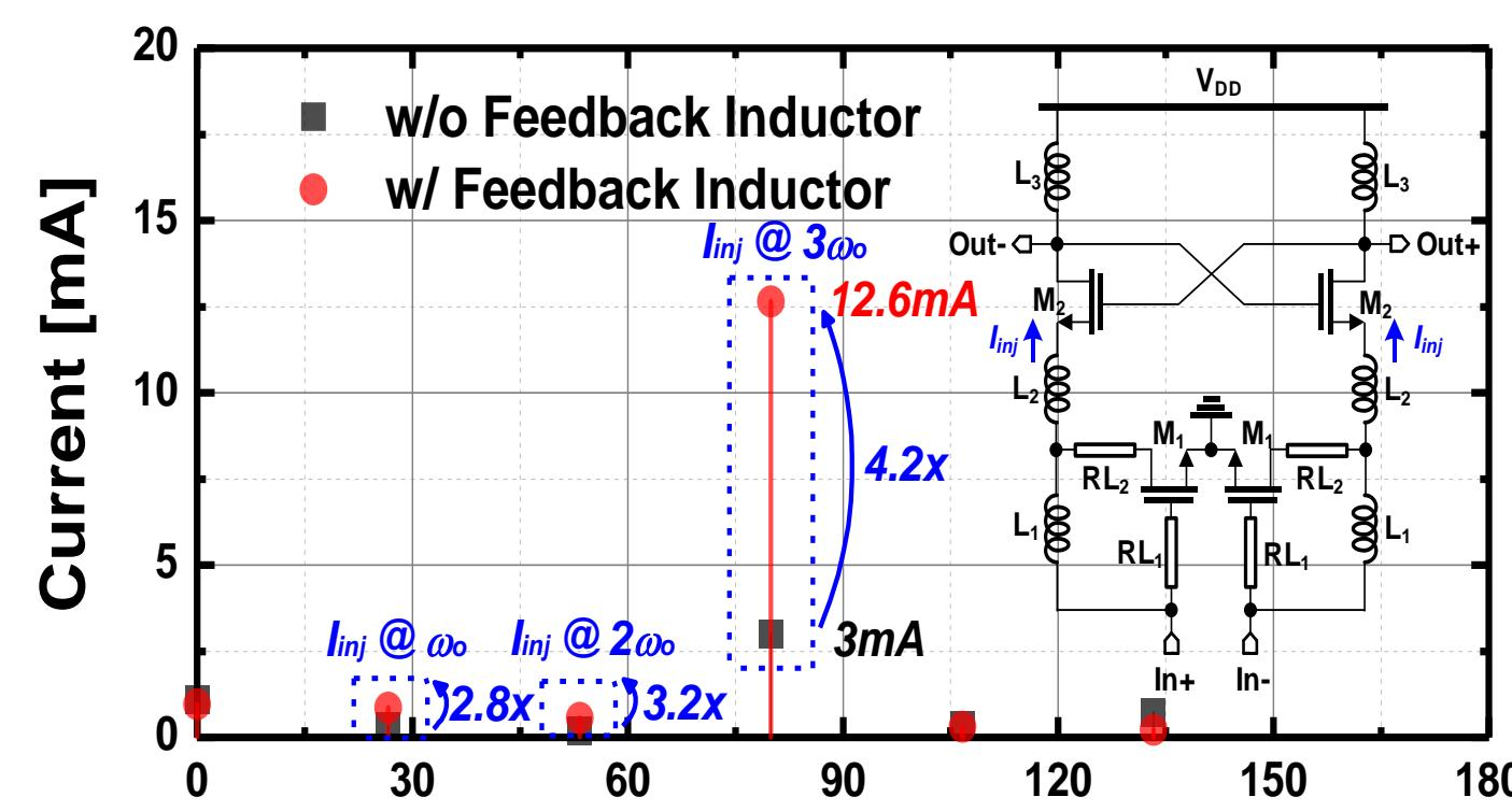
Fig. 5. Simulated injection current with and without feedback inductor for the proposed ILFD.
