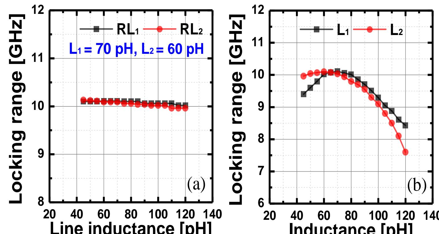
Fig. 3. (a) Locking range versus  $RL_1$  and  $RL_2$  with given  $L_1=70\text{pH}$  and  $L_2=60\text{pH}$ . (b) Locking range versus  $L_1$  and  $L_2$
