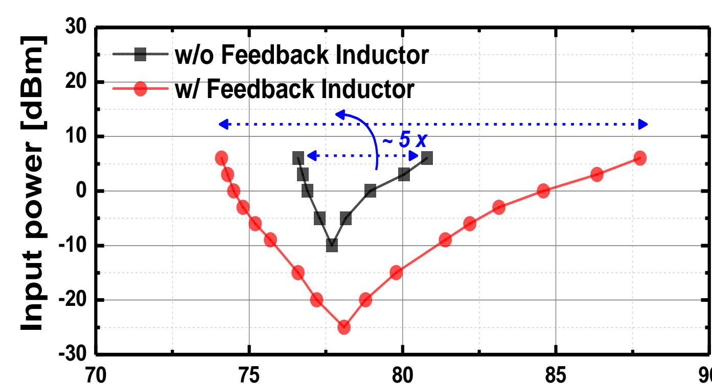
Fig. 6. Simulated locking range with and without feedback inductor for the proposed ILFD.
