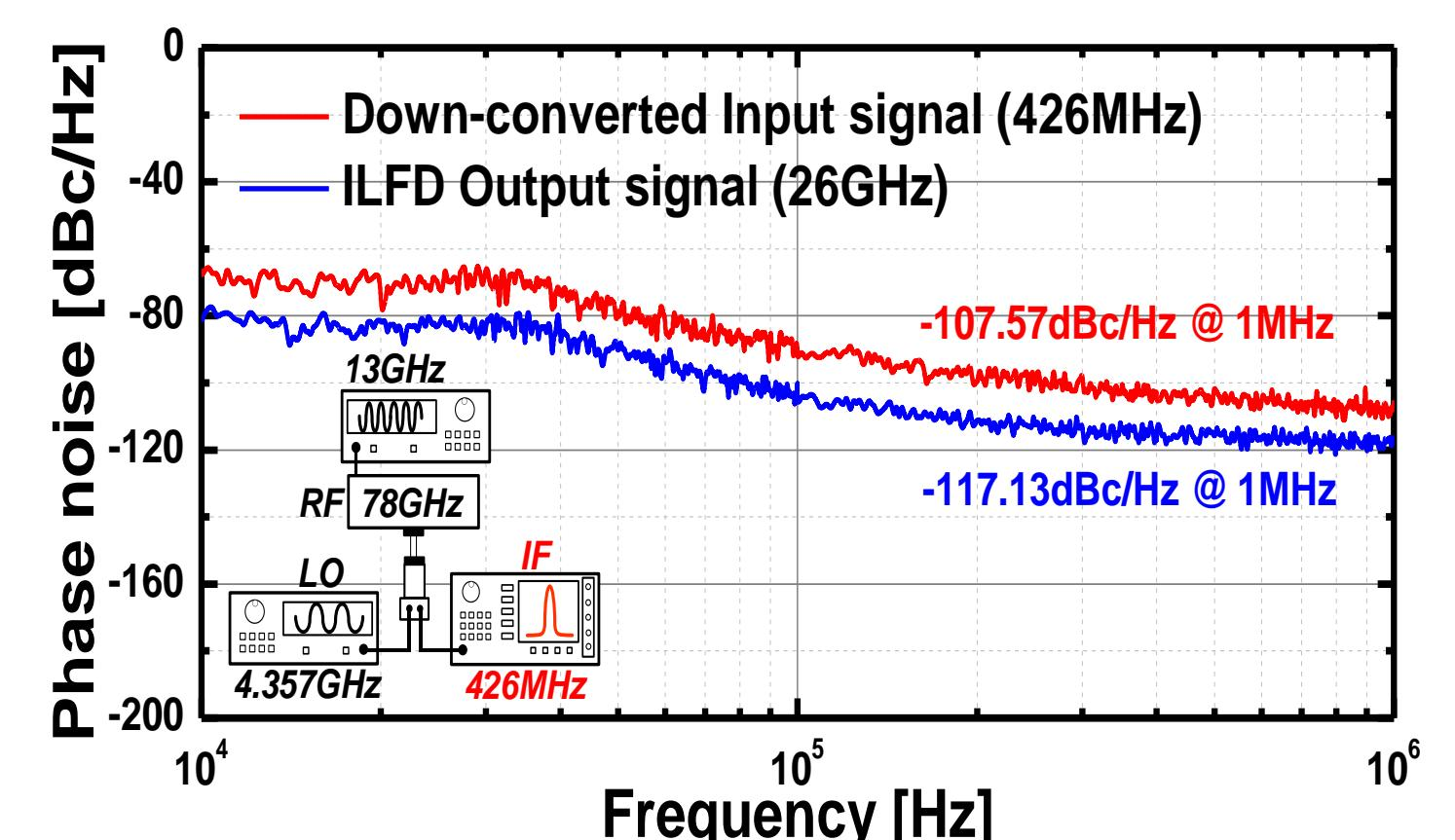
Fig. 12. Measured phase noise for the proposed ILFD in locking condition. The phase noise of the input frequency was measured using by harmonic mixer (Agilent 11970W).
