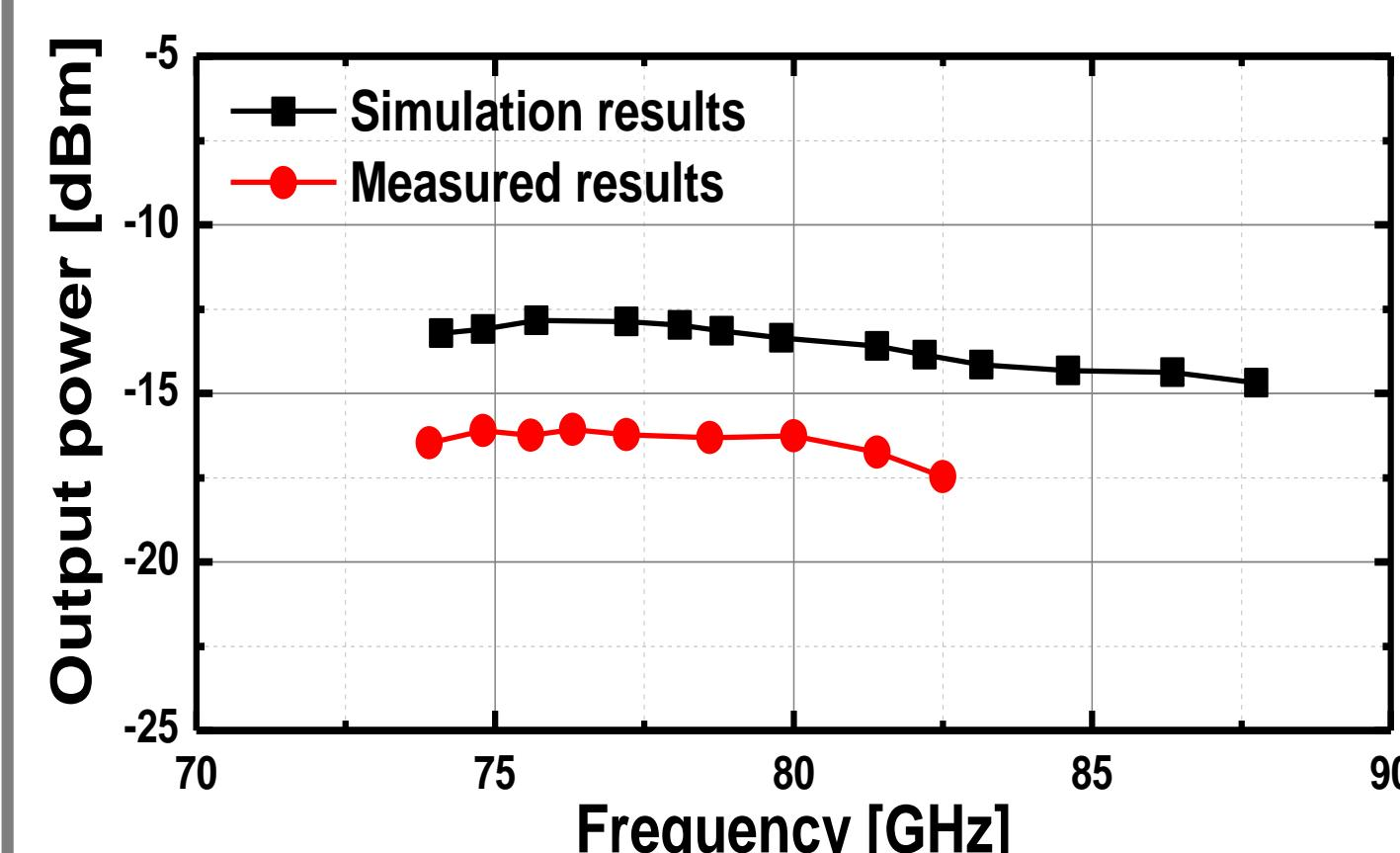
Fig. 11. Simulated and measured output power for the proposed ILFD with input power of 0dBm. The measured output power is considered the loss caused by probe-tip and cable.
